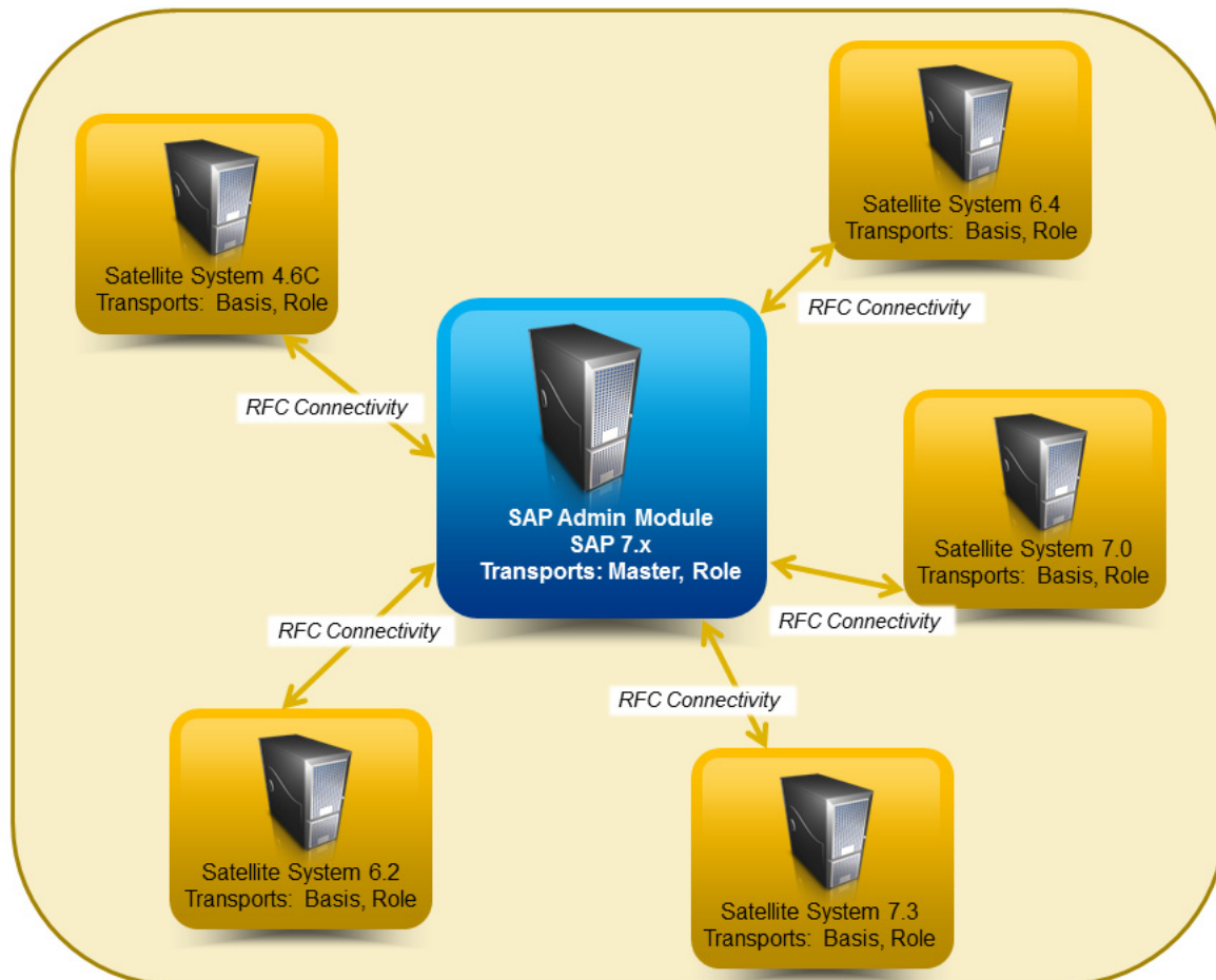
Figure 2: Transports for FlexNet Manager for SAP Applications in the SAP system landscape
